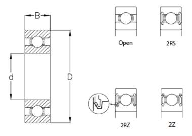
B = 12 Ball grade = 3 C (KN) = 9.95 C0 = 5 d = 20 D = 42 Max rpm. = 26000 Type = 6004
